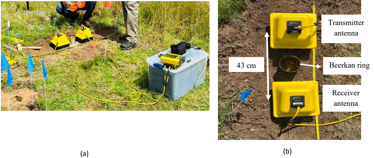
Figure. 3.1. Experimental set-up for the Beeken infiltration experiment and data collection using 500 MHz ground-penetrating radar (GPR) transducers. a) side view and b) top-down view.
