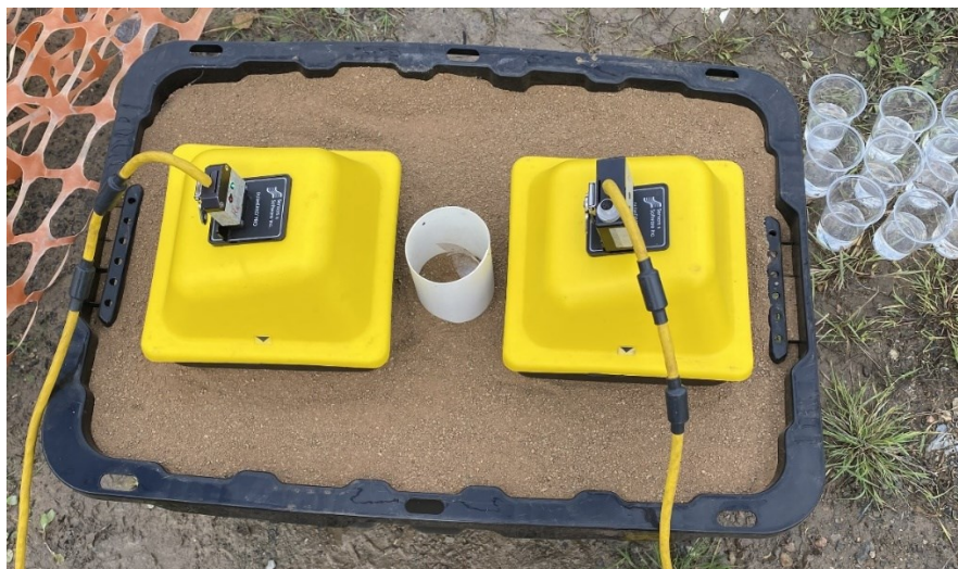
Figure 4.1. Data collection set-up for the Beerkan infiltration experiment monitored by ground-penetrating radar (GPR).
